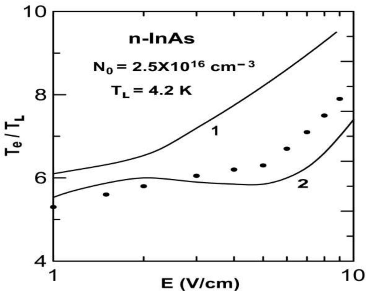
**Fig.1** Dependence of electron temperature upon electric field in n-InAs. Curve marked 1 is the result from the present theory and that marked 2 is the result obtained by Monte Carlo Method considering all the prevalent scattering mechanisms [6]. Symbols (•) represent the experimental data [14].
