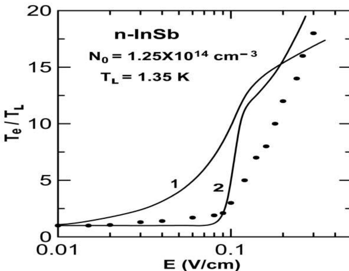
**Fig.1** Dependence of electron temperature upon electric field in n-InSb. Curve marked 1 is the result from the present theory and that marked 2 is the result obtained by Monte Carlo Method considering all the prevalent scattering mechanisms [6]. Symbols (•) represent the experimental data [13].
