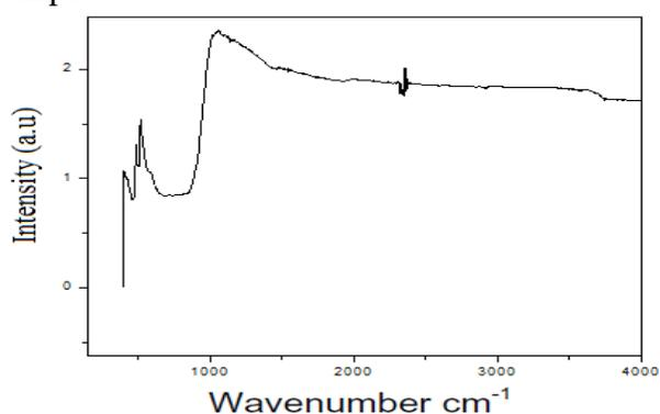
**Figure.2. Showing the FT-IR Spectra of the corundum sample collected from the study area.**
