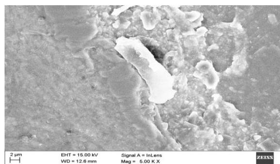
**Figure.3. The SEM image of the corundum sample collected from the study area showing Carbonates.**
