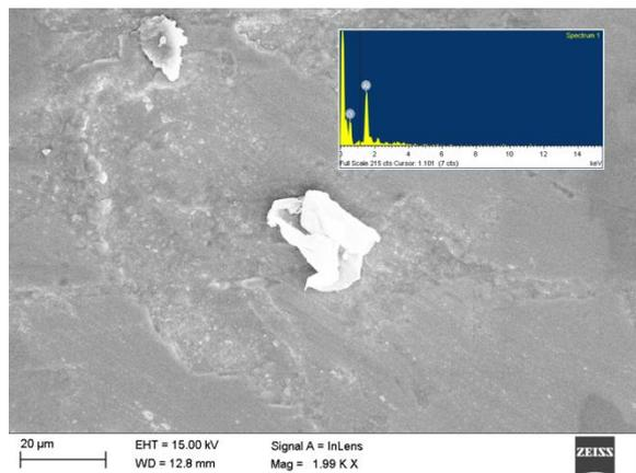
**Figure.4. The SEM image along with EDAX of the corundum sample collected from the study area showing hydroxylated form of Alumina.**
